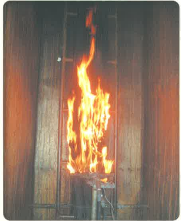
▲ During Fire Test (cable only)
